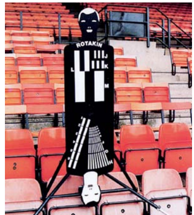
The Rotakin test, devised by the UK Home Office Police Scientific Development Branch, measures surveillance camera performance.
